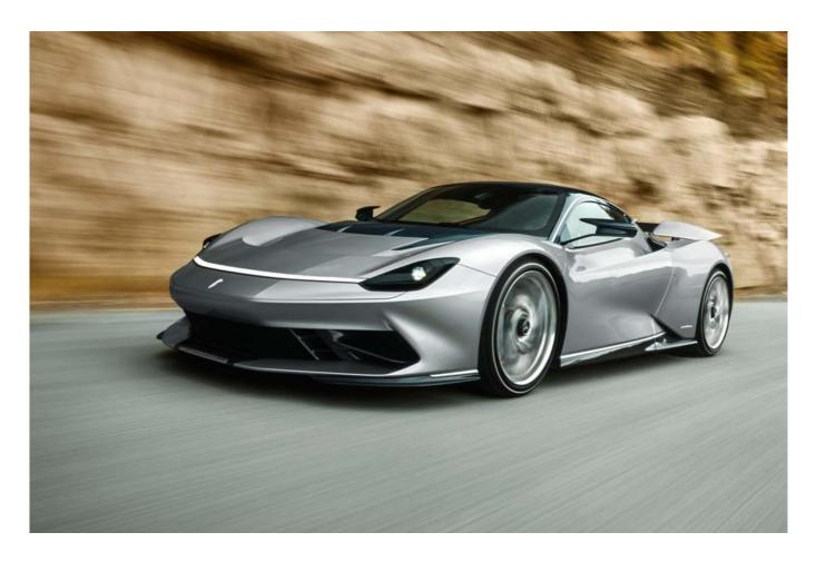
The Battista uses new battery technology to power 4 large electric motors giving four wheel drive and a power output of just over 1900 BHP. Some very fancy and expensive computer power controls wheelspin and both understeer and oversteer at the limit. As the limit is in excess of 200 MPH I doubt many owners will use it. Hats off to the Italians for daring to build a car that is on one hand environmentally friendly and on the other hand a car that upstages Ferrari, Alfa Romeo, and Lamborghini.
