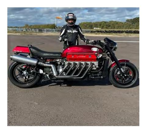
Brave or Mad? Motorbike with Viper V10 engine fitted Over 500 BHP and , in theory a top speed of 300 MPH.
