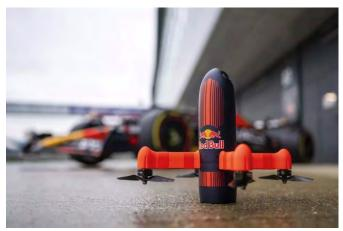
Capable of hitting speeds of 220mph this lightweight drone, developed by Dutch Drone Gods has a very short battery life when at full speed, only 3 minutes, however DDG are constantly updating and improving. Red Bull are currently in discussion with F1 and the FIA as to how this can be
