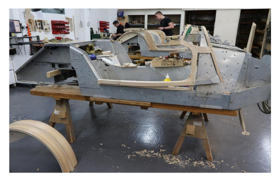
The shape of the car begins to emerge as first the ash frame is bonded to the platform.
